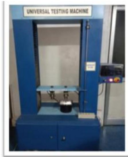
Figure 3: Universal testing machine
