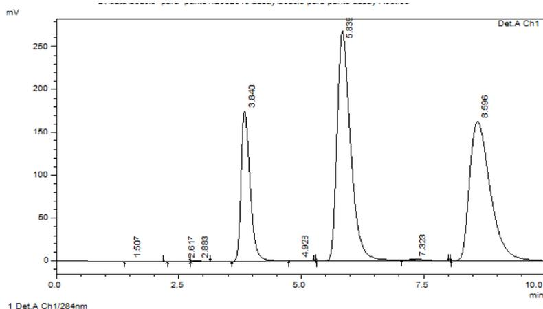
**Fig 4** chromatogram showing the combined standards of Paracetamol, Pantoprazole and Aceclofenac
