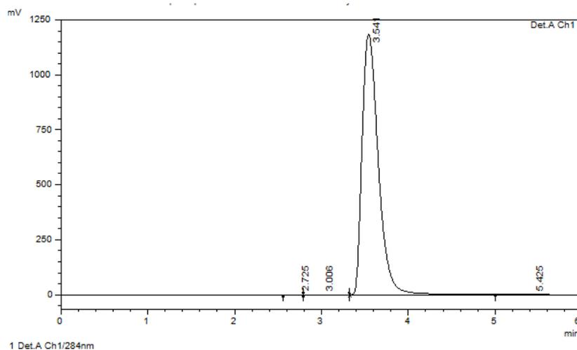
**Fig.1** chromatogram showing the retention time for paracetamol standard
