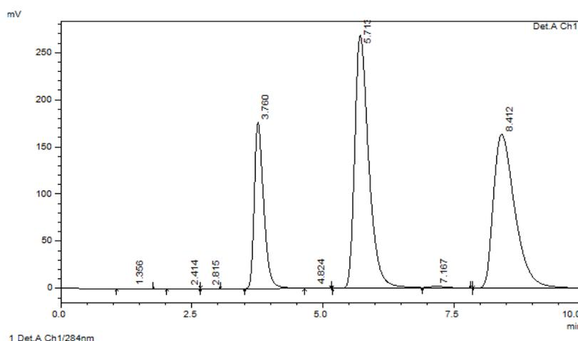
**Fig 5** chromatogram showing the combined formulations of Paracetamol, Pantoprazole and Aceclofenac
