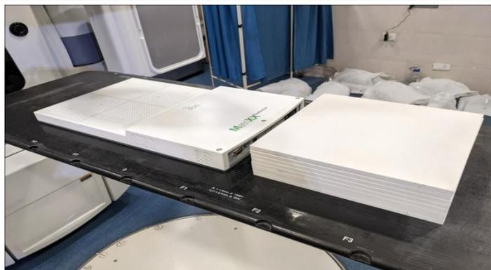
Figure: MatriXX Evolution ionisation detector array and RW 3 Slab Phantom
