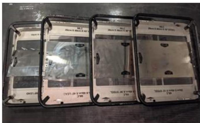
Figure: Physical Wedges of 15°, 30°, 45° and 60°
